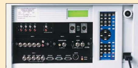
Rear view of Vista X5 showing LCD display panel and inset keypad
