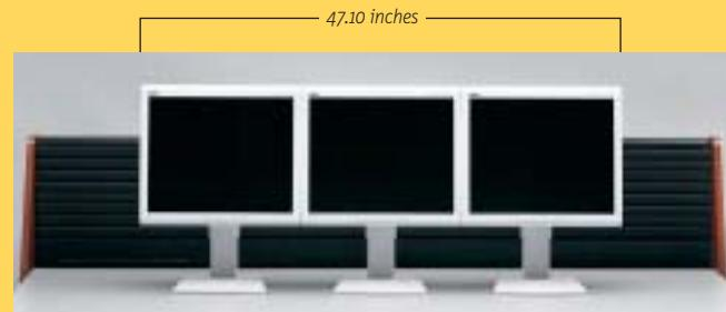
*With a thin-frame design that saves at least 12% horizontal desktop space compared to traditional LCD models, the MultiSync LCD1850X delivers a virtual single-monitor view in multiple-monitor environments.*
