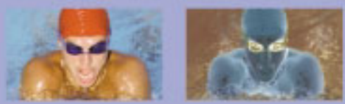
An Inverse mode will display inverted RGB values that will even the amount of wear on the screens phosphor.
