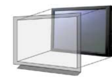
Other systems Because a screen is placed in front of the display, the image degrades due to parallaxing.
