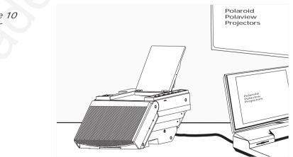
*The Polaview SuperPortable 10 LCD Projector in operation*  The projector has a monitor-interface connector that lets you view your computer video simultaneously on both the small and large screens.
