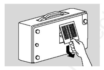
5 Remove the air filter and clean it with a vacuum cleaner. If dirt is hard to remove, wipe the air filter with a cloth moistened with water, then wipe it with a dry cloth.
