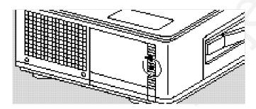
**4** Loosen the 4 lamp-assembly screws (you cannot remove them from the service door).
