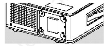
**Caution:** The lamp assembly gets very hot during operation. Use appropriate care when changing lamps. Make sure that the lamp assembly has cooled for at least 3 to 5 minutes before touching it.
