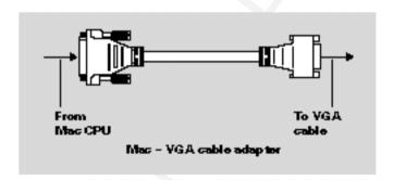
Use the cable adapter and supplied VGA video cable to connect the projector to your Macintosh computer.
