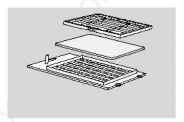
6 Reassemble and re-install the air filter.
