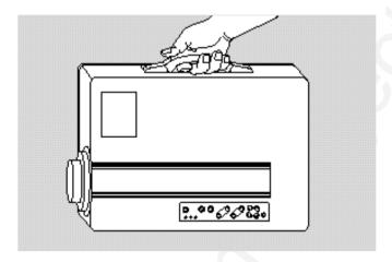
If you are moving the projector a short distance, grasp the sides of the projector securely, as shown below, to stabilize the weight of the unit.
